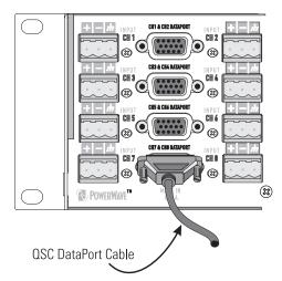
Connect to the DataPort using a QSC DataPort cable. Align the connector with the socket housing and insert fully. Finger-tighten the retaining screws.
